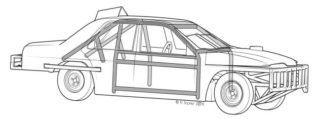
• It is required to have a minimum of two rearward supports going back from the top of the rollcage hoop down to the chassis – one on each side of the car (see diagram). You may run the rearward supports in a criss-cross fashion, running diagonally from the top of the rollcage hoop at the driver's side to the chassis on the passenger side and vice-versa.
